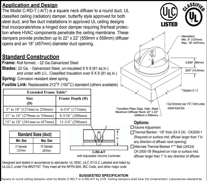
Square to round ceiling dampers shall be Model C-RD-T or C-RD-A/T by CVS. Ceiling dampers shall bear the Underwriters' Laboratories labeland be rated for both steel duct and flex duct installations. No external damper supports shall be required for ceiling dampers up to and including 18" (457mm) diameter. Ceiling dampers shall be of the non-asbestos type and be furnished with a fusible link volume controller where shown (Model C-RD-A/T).
